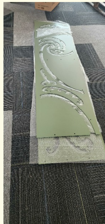
Laser cut Maihi panels to be installed on the front of the Whare.
